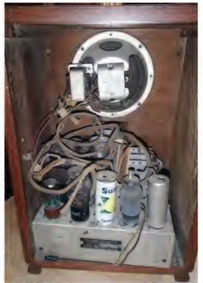
Someone replaced an IF transformer on this 1935 Rogers radio with a juice can.
